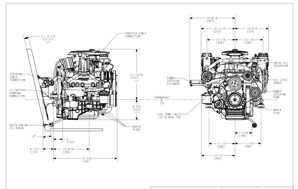
DRW43-004 SHEET 1 OF 2 4.3L MPI ALPHA MULTI-POINT DRAIN UNIT OF MEASURE in. (mm)
